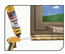
**Tekapur Low Expansion** gun grade is a one-component polyurethane foam hardening by air humidity. Thanks to its special formulae, this foam has a very low expansion and is thus particularly suitable for gluing, fixing and sealing.
