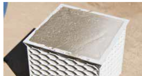
Wait until the specimen is fully cured for testing (28 days).
