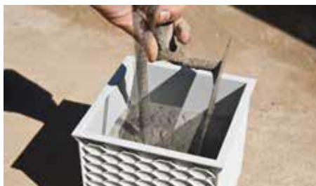
Fill completely, as specified, with the concrete to be tested.
