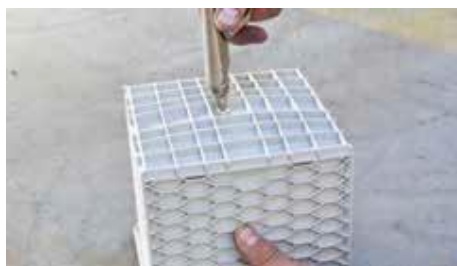
To extract the specimen, use a jet of air from the hole previously plugged.
